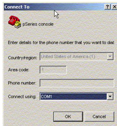
Figure 2-3 HyperTerminal: choosing the serial port
